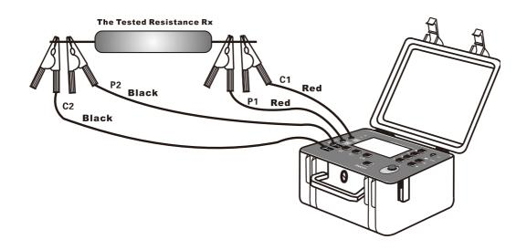
The figure below shows the equipotential resistance between the meter box and the ground and the lower line.
