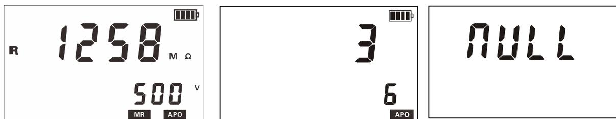
In the data review state, press and hold the “MEM” key to enter the data deletion, press “▲” or “▼” to select “NO” or “YES”, select “NO” and then press “SET” key to not return to the data review state. “YES” Press “SET” again to delete the stored data. After deletion, the following figure is displayed.
